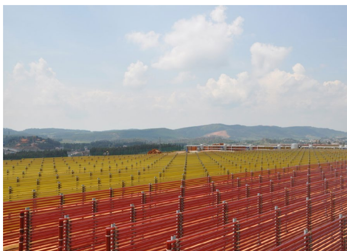
Figure 8. BGG's 100% Glass Tube Photobioreactor Production System
